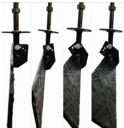
Fig. 3. Tuproq surgichlarning vertikalga nisbatan 30, 35, 40 va 45° burchak ostida o'rnatilishi / Fig. 3. Installation angle of soil pushers relative to the vertical at angles of 30, 35, 40 and 45°
