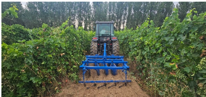
Fig. 4. Tekislagich bilan jihozlangan dala qurilmasining ishchi ko'rinishi / Fig. 4. Working view of a field installation equipped with a leveler
