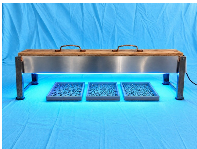
Fig. 2. General view of the UV treatment stand
