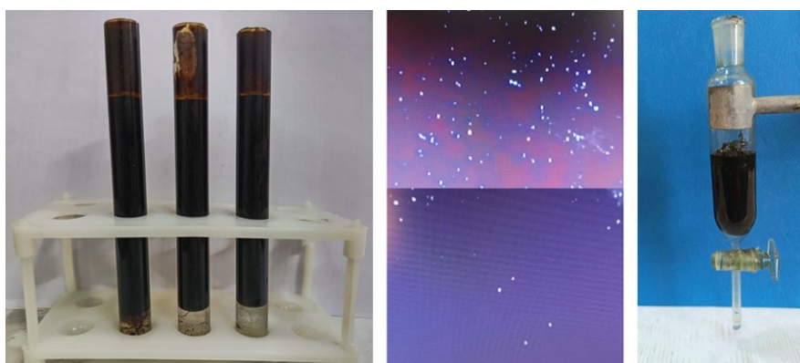
Fig. 4. Demulgator qo'llanilgan neftning tashqi ko'rinishi: A — sinov probirkalari; B — emulsiya namunasi; C — suvni ajratish kolbasi / Fig. 4. Appearance of oil with the demulsifier applied: A — test tubes; B — emulsion sample; C — water-separating flask
