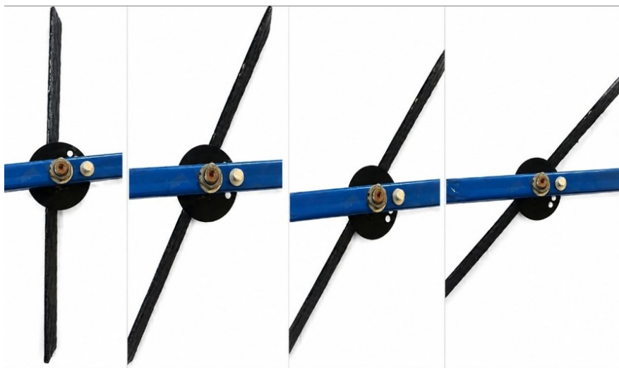
Fig. 2. Tuproq surgichlarni harakat yo'nalishiga nisbatan 25 (a), 30 (b), 35 (c) va 40° (d) burchak ostida o'rnatish / Fig. 2. Installation of soil pushers at angles of 25 (a), 30 (b), 35 (c) and 40° (d) relative to the direction of movement
