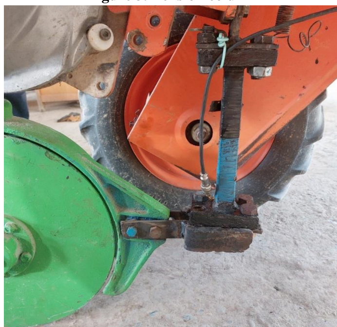
Figure 4. A view of tension column as it is installed in a laboratory-field device
