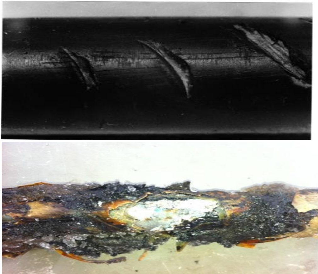
Figure 1. Damage to the insulating sheath and aluminum sheath of the power supply cable.
